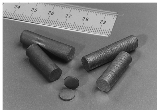
Fig. 1. Cylindrical specimens and disks from Ringsdorff EK98 graphite (darker) and CFC (metallic appearance, striated) obtained from virgin JET graphite tiles.
